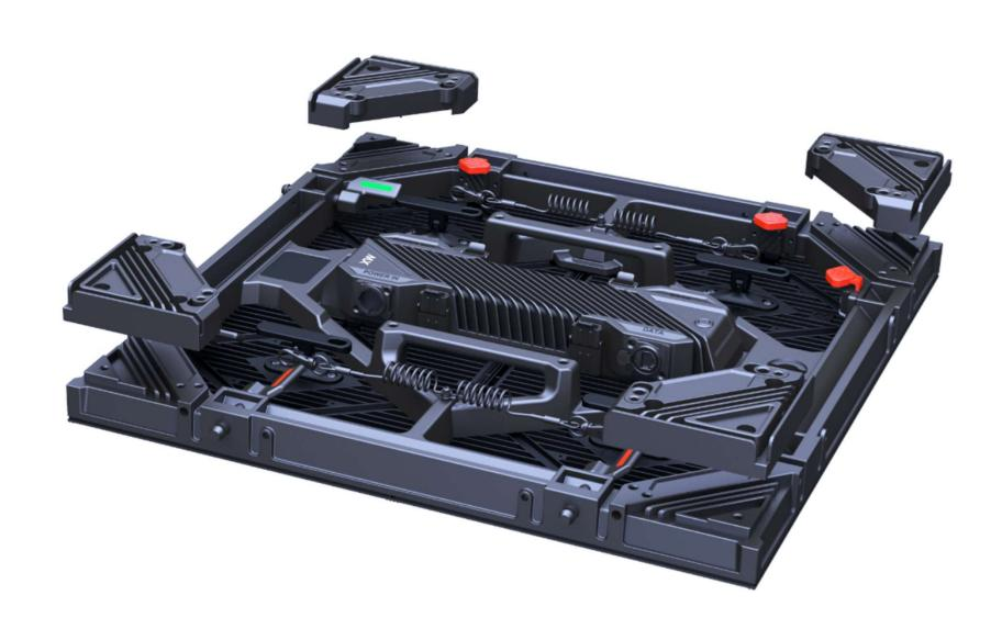
Slide block can move M6 and M8 hole. M6 screw hole use to connect 55mm frame; M8 screw hole use to connect 62mm frame.
